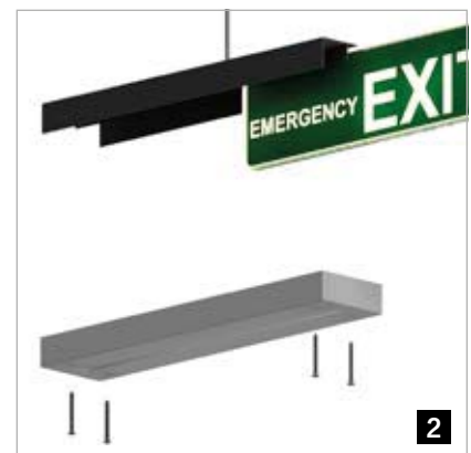
Pair of panes is inserted from the side
